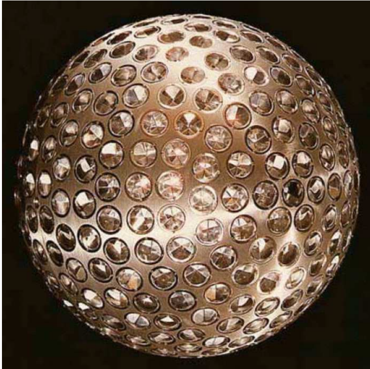
Fig. 2.8. The LAGEOS-1 satellite (identical to LAGEOS-2). Dedicated laser ranging satellites have a long-term orbital stability because of their spherical shape and high mass-to-area ratio.
