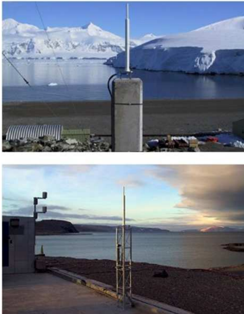
Fig. 2.18. Illustration of two DORIS stations. The stations are Rothera, Antarctica (top), and Thule, Greenland (bottom).
