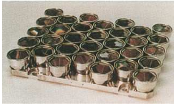
Fig. 9.4. Retro-reflector arrays on GPS-35 and GPS-36 satellites.
