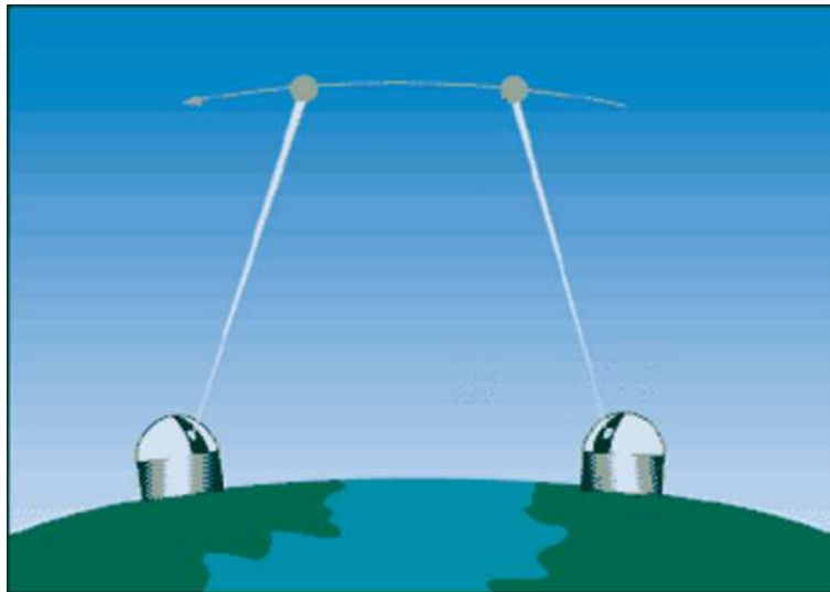
Fig. 2.7. Principle of satellite laser ranging.
