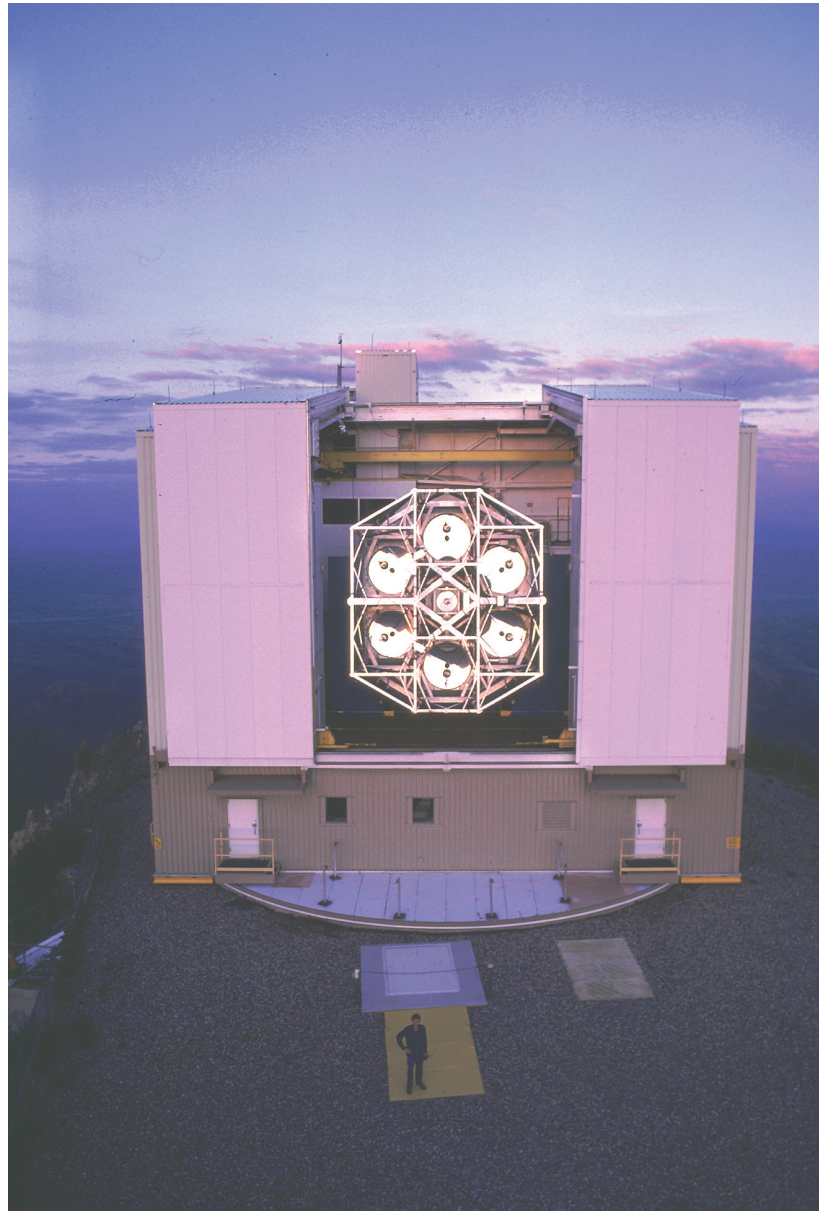
FIGURE 3.3 The six 1.8-meter-diameter mirrors that until 1999 composed the primary mirrors in the (old) Multiple Mirror Telescope (MMT). These mirrors now in storage are proposed for use in the CSS+ (see text). SOURCE: Courtesy of the MMT Observatory.
