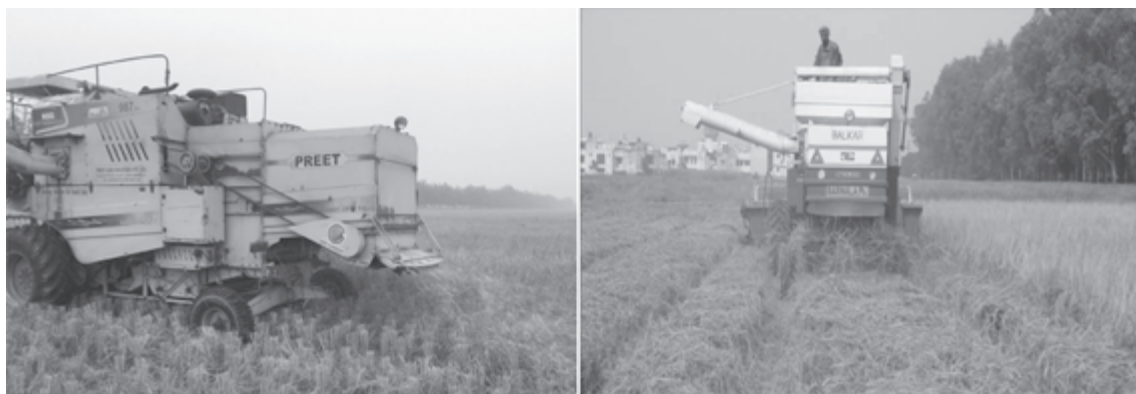
Fig. 1. Super SMS (left) and SMS (spreader on right) while harvesting rice
